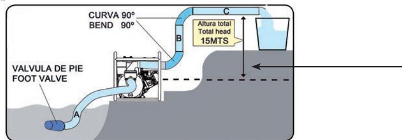
We need to transfer water from a raft to a tank located 15 meters of an elevation. The main line is a PVC hose 35 meters long (A+B+C). Two curves and a foot valve complete the installation.
