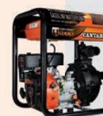
**Salt water or chemicals:** Body, volute and turbine have been manufactured in polypropylene replacing classic metals. It can be used with salt water or low level of aggressiveness chemicals, such as fertilizers. It's not valid for transferring oils, fuels, high aggressiveness corrosives and high viscosity liquids or with high levels of adherence.
